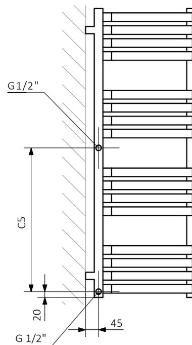
A – Height B – Width C1-C5 – Distance between pipe centres D – Horizontal distance between mounting bracket centres
