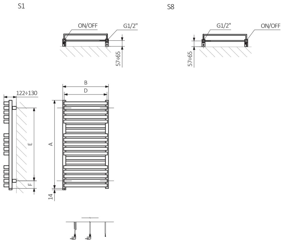
A – Height B – Width C1-C5 – Distance between pipe centres D – Horizontal distance between mounting bracket centres
