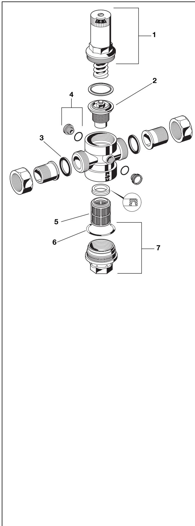
**Spare Parts****Pressure Reducing Valve D06F, from 1997 onwards**
