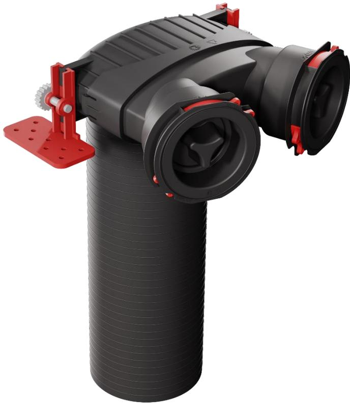
The plenum box with OneClick technology® allows the connection of up to 2 90mm ducts to a 125 mm supply / exhaust air diffuser. Factory-assembled, complete with a set of plugs and gaskets. Leave unused slots blanked. Constructed from high quality polypropylene.
