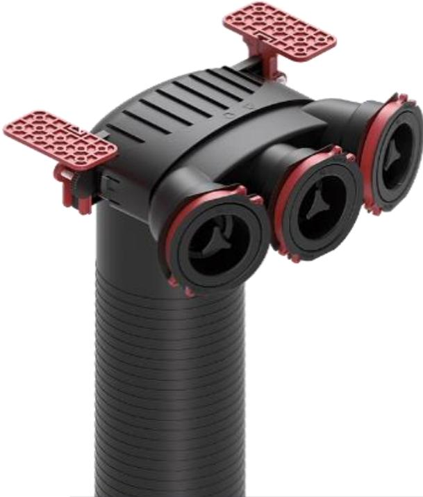
The plenum box with OneClick technology® allows the connection of up to 3 75mm ducts to a 125 mm supply / exhaust air diffuser. Factory-assembled, complete with a set of plugs and gaskets. Leave unused slots blanked. Constructed from high quality polypropylene.
